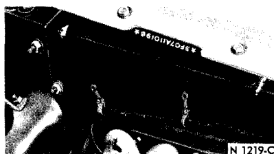
FIG. 5—Vehicle Identification Number Location—Comet, Falcon and Mustang
