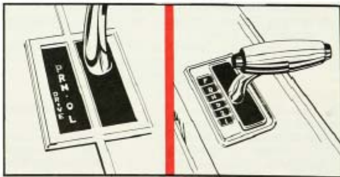
Figure 2—C6 Transmission Selectors: Automatic (L) Fairlane Sports-Shift (R)
